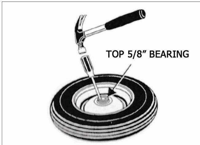
The fourth step is to remove the 5/8” bearing, should this be required. This can be done by tapping the back side with a screwdriver and hammer. Be sure to move the screwdriver around the bearing to avoid binding as much as possible.
