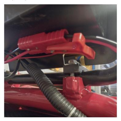
With these disconnected, the lower point, coming from the battery pack, connects straight to the battery charger.
