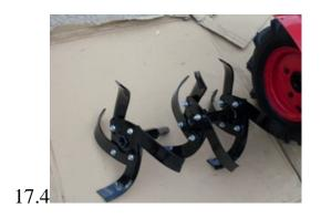
Picture shows tines with end protection discs attached with 2 and 3 sets of tines on shaft. To attach tines to machine revert to paragraph one of these assembly instructions.
