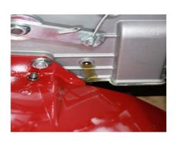
15. Fill the Engine with oil up to the top of the threads in the filler hole using a small funnel. Use 15–40 sae
