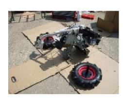
6. Tilt one side of the machine up at a time and slide wheel onto axel lining up the hole in the drive shaft with the wheel spigot, insert clevis pin and retaining clip, repeat for both wheels.
