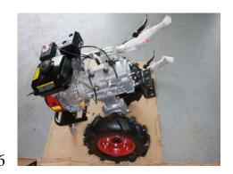
7. Locate handlebar frame and remove 2 x retaining bolts, these should only be hand tight, position the frame over the gearbox and insert bolts through frame and rubber mountings on the same side as oil filler cap. (As shown) apply loctite thread seal (not supplied) attach nuts tighten up fully so there is no movement. 14 +16mm spanners required.
