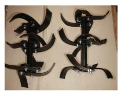
Note the inner bolts face away from the drive shaft housing so as not to foul it when moving. (loctite id to be used on all bolts, not supplied).
