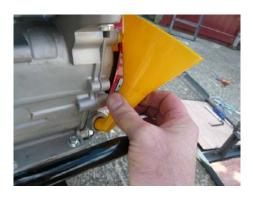
**16.**Put some oil in the Air filter oil bath use 15 -40 sae oil up to the **mark** shown on clear outer cover
