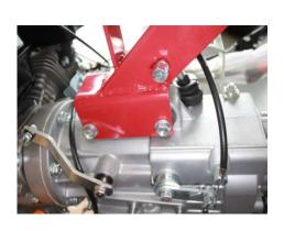
8. Remove protective wrapping from boss on handlebars & slide adjustable rotating collar onto bolt as shown.
