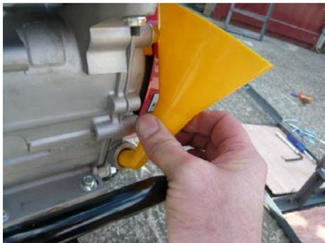
16. Put some oil in the Air filter oil bath use 15 -40 sae oil up to the **mark** shown on clear outer cover
