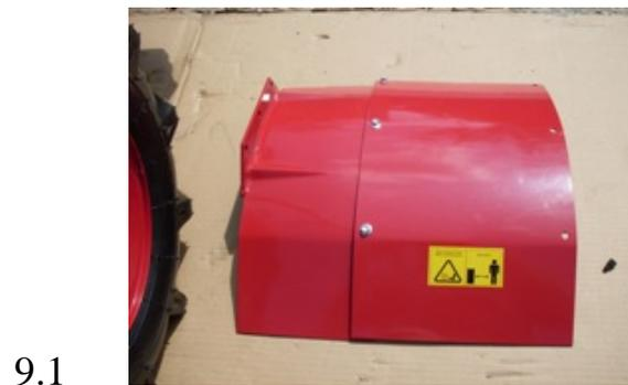
10. Bolt R/Hand & L/Hand mudguards on to machine using a 13MM spanner, (use loctite on all nuts not supplied)
