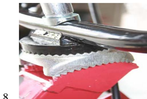
**8.1 Install handlebars – 8.2 (noting position of R/Hand cable to run on the underside of frame)**
